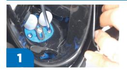
Remove the 3 dimensional equalisation system. Unscrew the top two regulator screws from the inside of the mask on the orinasal plate (Torx T20 screwdriver).
