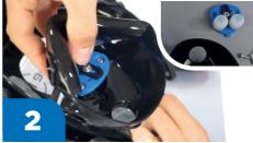
Carefully disconnect the Orinasal pocket from the communication port.
