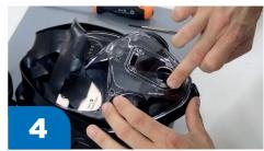
Check and clean the regulator O-ring in the visor.
