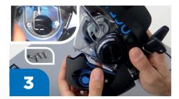
Unscrew the two lower regulator screws Remove the NEPTUNE III 2nd stage regulator from the mask (Torx T20 screwdriver).
