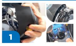
Install 2nd stage regulator: Begin to connect the center of the exhaust deflector to the exhaust deflector retainer. Align the regulator on the visor making sure all orientation points are appropriately in position, the front O-ring is fully covered, and the four regulator screw holes are in alignment with the holes in the visor. There should be no space left between the regulator and the visor. Screw in the two lower regulator screws first.
