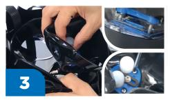
Install the orinasal pocket with the orinasal plate in position and line up the upper regulator screw holes so the two screws will easily fall into the threads of the regulator body. Use the two top screws to keep the orinasal plate and orinasal holes aligned.
