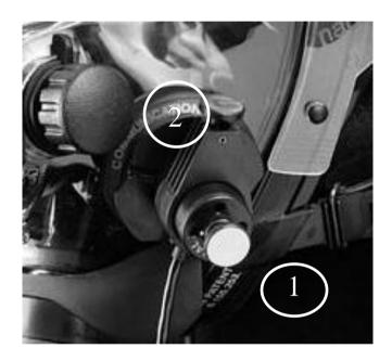
Pressing the volume button (2) and keeping it pressed you hear a sound growing in intensity. This sound level indicates of the speaker volume. When the sound reaches the maximum level (after a few seconds) it starts to decrease until it reaches the minimum level and up again until the button is released. When you release the button the volume is adjusted at the desired level.
