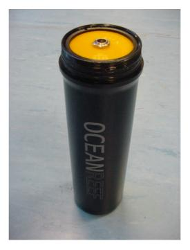
Batteries are protected by a black anodized anticorodal housing, with an overpressure valve to prevent explosions in case of battery malfunctioning. There are 8 rechargeable ni/mh batteries, total 9.6 volt 4 A/h. The jack connector that connects the battery to the main unit is designed to let you screw the two parts together without any other operation.
