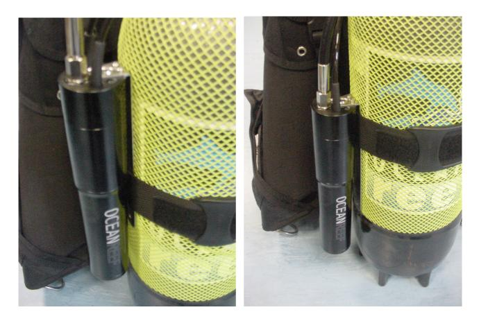
Screw the HP hose to the HP sensor on the main unit and to the HP port on the first stage.
