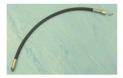
HP hose must be screwed on one side to the HP sensor, and on the other side to the HP port of the first stage.
