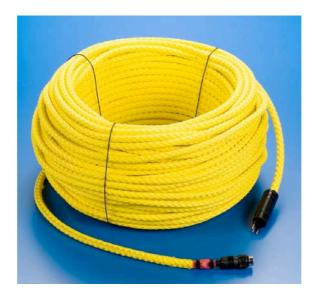
1xmini rg59 + 4x0.18mm<sup>2</sup> cable with a polyurethane jacket to better resist to salt water. The whole cable is covered with a rope made to resist to 4000N pull strength.
