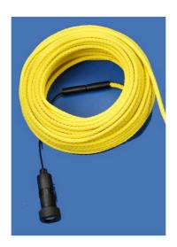
The cable is a mini RG59 + 4x0.18mm<sup>2</sup> cable with a polyurethane jacket to better resist to salt water. The whole cable is covered with a rope made to resist to 4000N pull strength.
