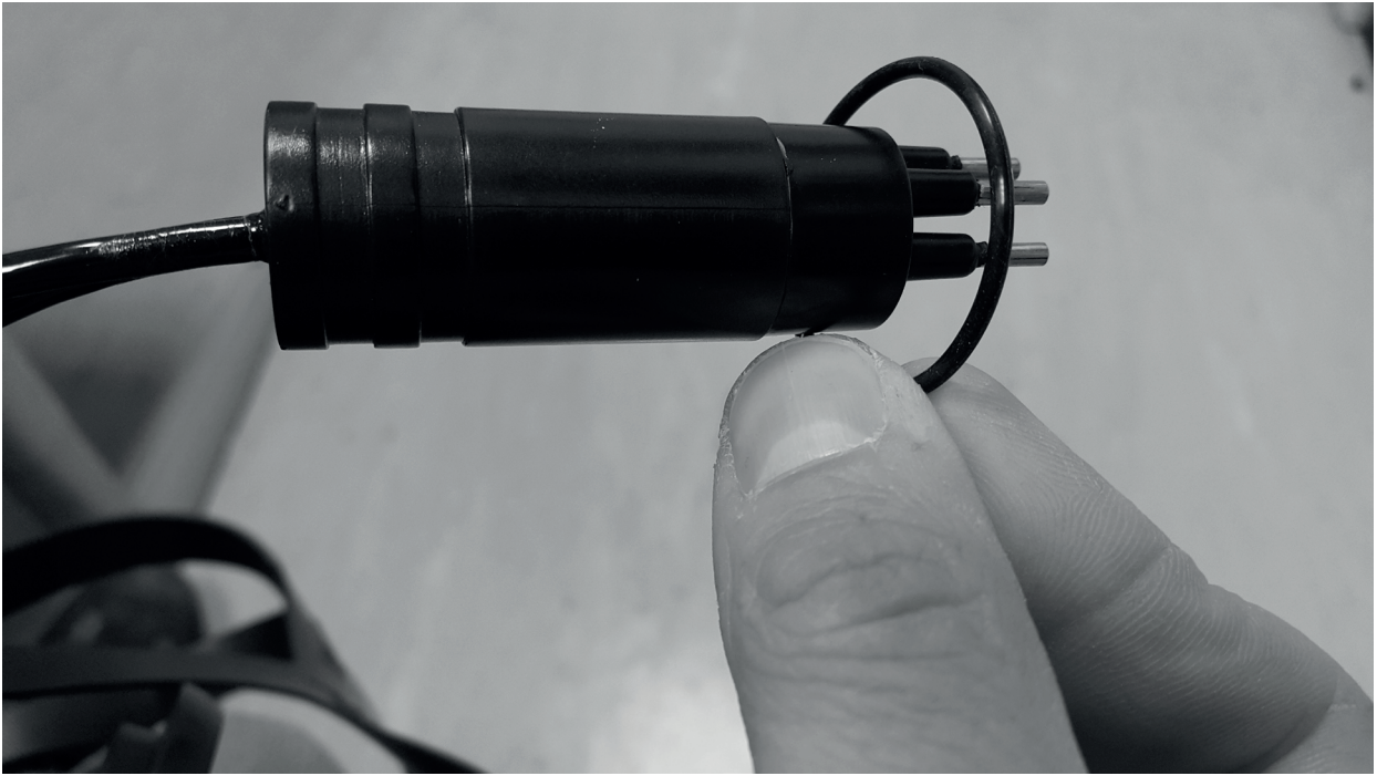
Hold cable in place with 3d Oring - as shown.
