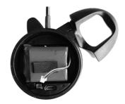
The polarization of the plug has an orientation. Do not force it if it is hard to push it down.
