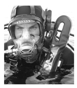
The GSM VHF is a very unique communication system with the integration of Ultrasonic / Underwater communication features and the VHF long distance communication requirements. It is mainly dedicated to Rescue Team Divers and was developed thanks to the collaboration with the Italian Red Cross.
