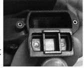
When the battery has been installed, check that the battery housing and O-ring are clean. The O-ring must always be lubricated with a thin layer of silicone lubricant.
