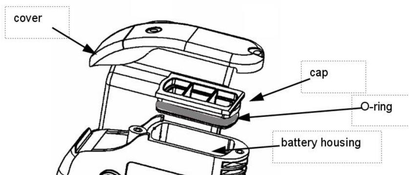
When the battery has been installed, check that the battery housing and O-ring are clean. The o-ring must always be lubricated with a thin layer of silicone lubricant.
