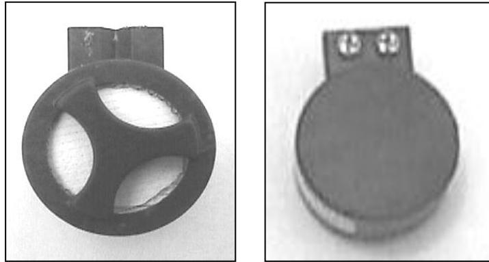
The GSM DC use a dynamic microphone, "D-Mic" encapsulated and protected by a hydrophobic membrane.
