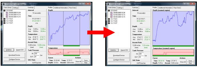
Under **Tank Pressure**, enter your in and out tank pressures and your SAC will be calculated in Bar or PSI per minute.
